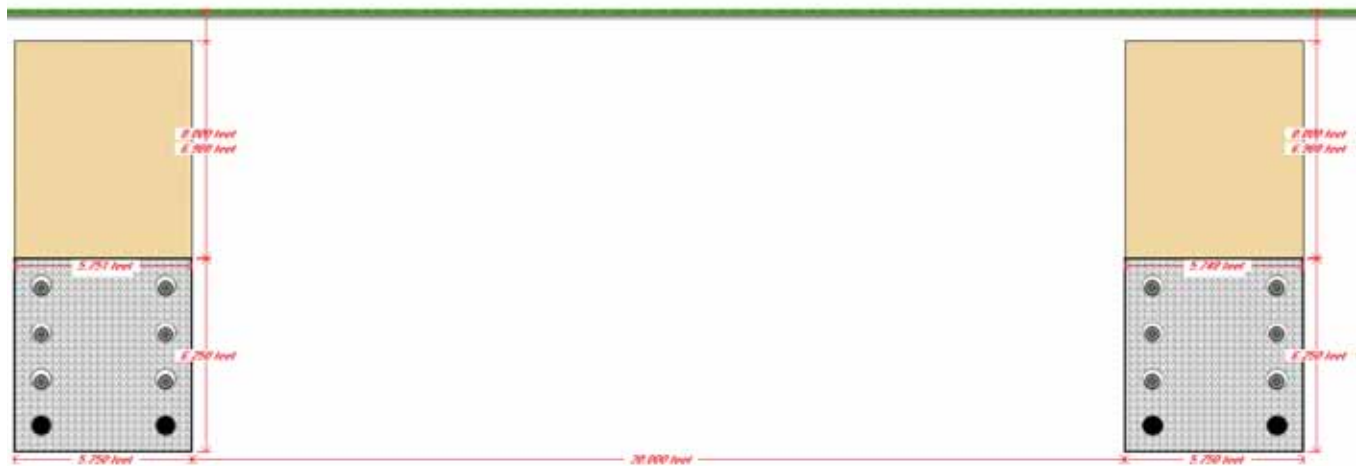
Figure 5 500-kV Duct Bank Configuration with Four Cables per Phase, 85% DLF
