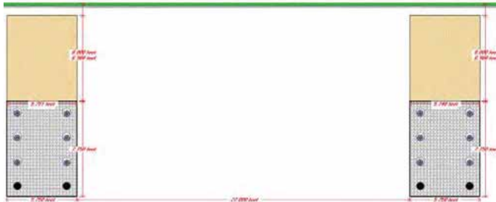
Figure 4 500-kV Duct Bank Configuration with Four Cables per Phase, 100% DLF
