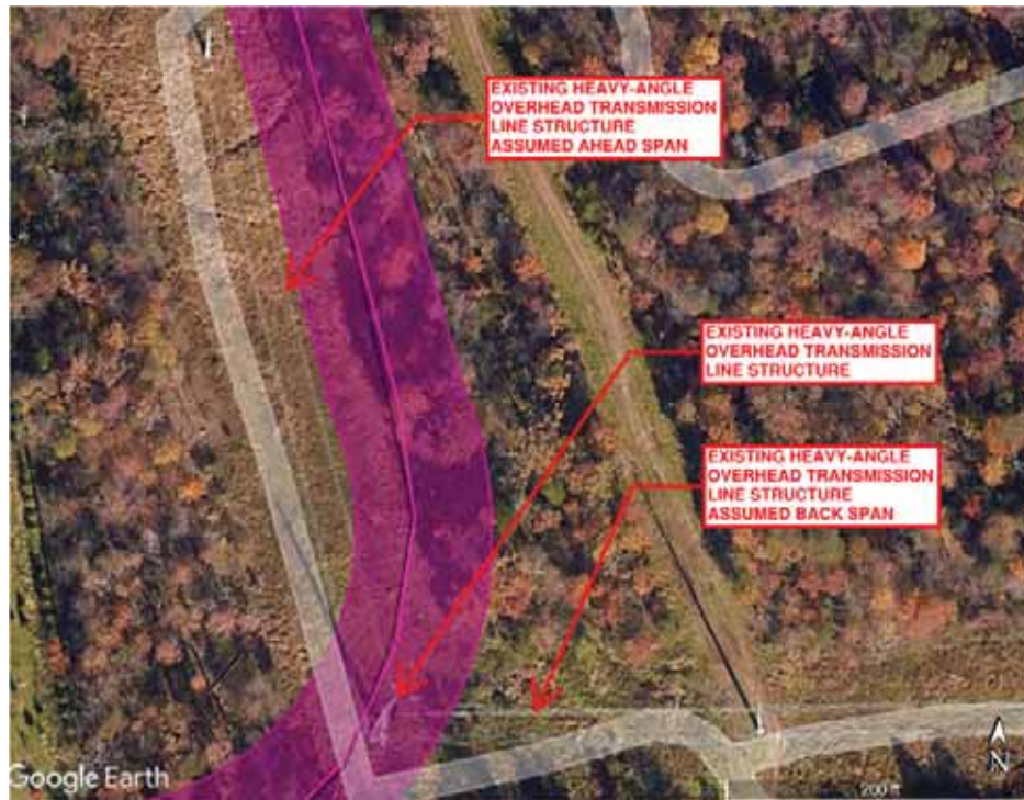
Figure 4-63 UG Route R4 Crossing with Existing Heavy-Angle Overhead Transmission Line Structure
